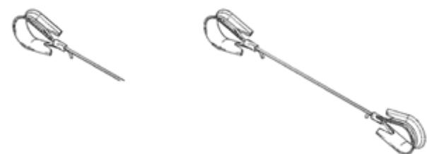
The thimbles provided in the 160001-01 installation kit can be used with the loop sleeve or copper sleeve to produce very rugged displacement cable terminations or leaders for attachment of the position transducer to the application. See Figure 11.
